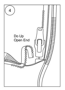
4. Take a new runner and thread it on the top end of the zip, this is the side with the zip stop at the bottom.
