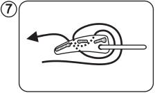
Cross section view of how the cam band should be threaded through the cam buckle.
