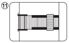
After securing the cylinder, check that the belt is sitting straight and firmly.
