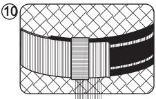
If mesh is used on the cylinder, part it to allow the cam band to grip on the cylinder paint surface.
