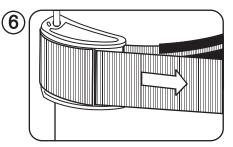
To finally clamp the cam buckle, pull on the webbing to make the buckle snap over.
