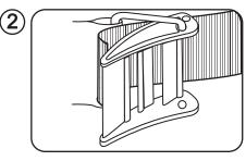
Before threading the buckle turn it back against the metal loop. o re-thread the buckle start by pulling the webbing through the metal hoop.
