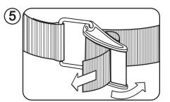
Secure the webbing by pulling the buckle slightly forward. Now thread the remaining webbing through the buckle as shown.
