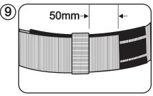
Once secure, the webbing is then velcroed down and tucked under the webbing loop,leaving 50mm (2") spare.
