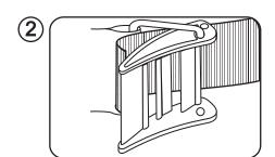
Before threading the buckle turn it back against the metal loop. o re-thread the buckle start by pulling the webbing through the metal hoop.
