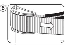
To finally clamp the cam buckle, pull on the webbing to make the buckle snap over.
