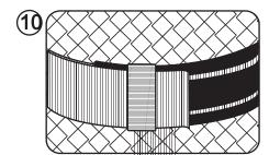
If mesh is used on the cylinder, part it to allow the cam band to grip on the cylinder paint surface.
