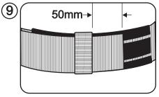
Once secure, the webbing is then velcroed down and tucked under the webbing loop,leaving 50mm (2") spare.
