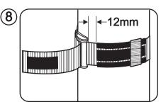
Ensure that the rubber sleeve does not interfere with the buckle.
