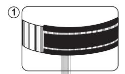
Ensure the rubber sleeve aligns with the velcro.
