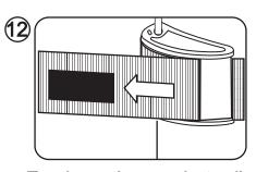
To release the cam, just pull on the webbing. The belt can be slid off and on the cylinder without re-adjustment.
