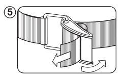
Secure the webbing by pulling the buckle slightly forward. Now thread the remaining webbing through the buckle as shown.
