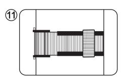
After securing the cylinder, check that the belt is sitting straight and firmly.
