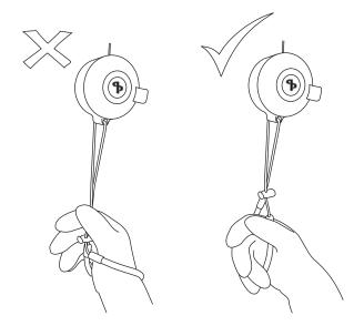
When using the reel with SMBs do not secure around wrist whilst inflating. Holding the strap in the palm of the hand allows instant release if required.
