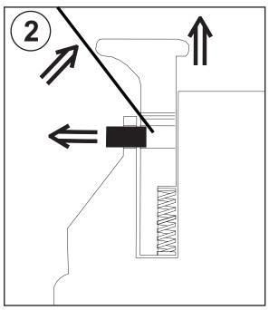
Once the pin is showing, pull the Lock Pin out with small pliers and remove the Spool Stop.
