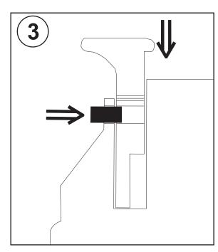
Remove the two springs from the recesses. Replace the spool stop and Lock Pin.
