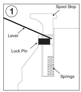
Using a small lever (e.g. needle or jewellers screwdriver), push out the Lock pin.
