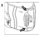
Showing CORRECT loading of pouch with flap tucked under outer edge top & bottom
