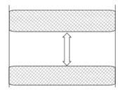
2. If mesh is used on the cylinder, part it to allow the cam band to grip directly on to the surface of the cylinder.
