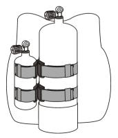
**Note:** The top cam bands fit through the BC Backplate and around the cylinders. The lower bands only go around the bands for stability.
