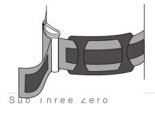
11. Once secure, the loose end of the webbing is then velcroed down and tucked under the webbing loop, leave 50mm (2") spare.
