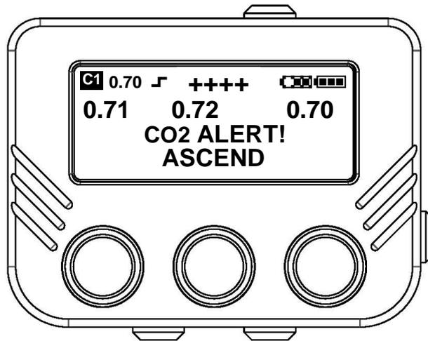
The CO<sub>2</sub> Sensor will trigger an alarm when CO<sub>2</sub> reaches 5mbar in the breathing loop. The display will show “CO<sub>2</sub> ALERT! ASCEND”. This will cycle with any other warnings that might be present. The warning will also be shown on the Vision HUD, whilst the buzzer sounds. The HUD will show solid red lights on both controllers for the period that the CO<sub>2</sub> is above 5mbar.
