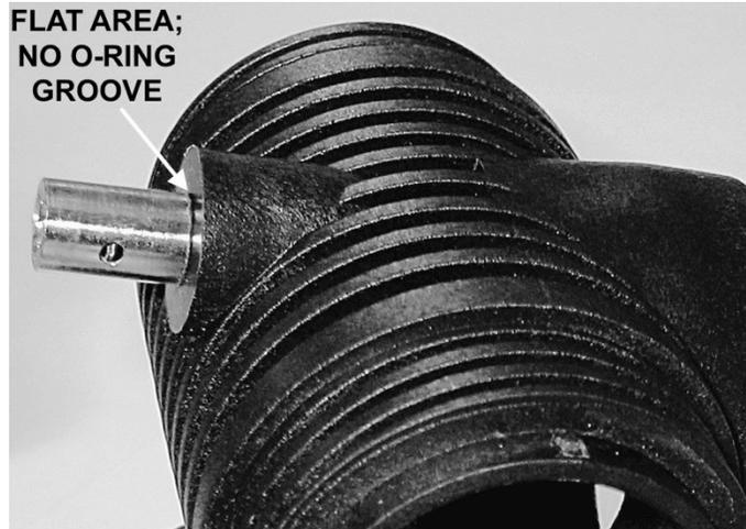
Pre-2006 (old) T-piece body: flat area around protruding shaft, no O-ring
