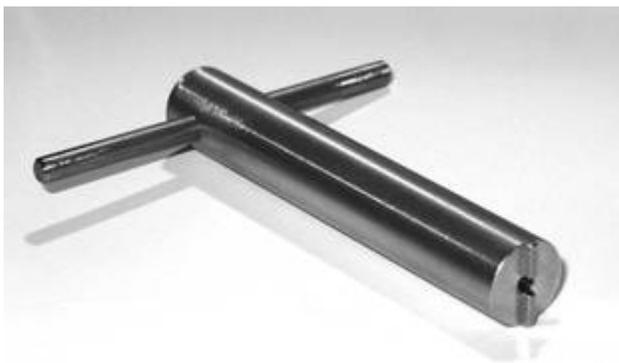
This tool is used for removing the tilt boss from the ADV body during disassembly, and screwing it back into the ADV body during assembly. Using this tool avoids damaging the delicate tilt boss and the inside of the ADV body.
