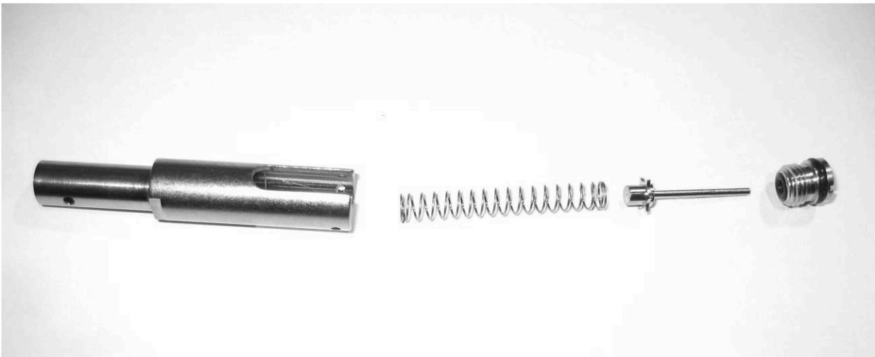
After removal check again if the tilt axle hasn't got bent by the removal process.
