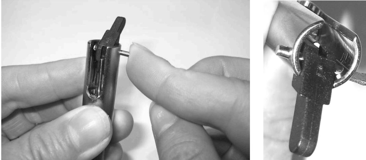
The pin holds its position in the lever solely by friction; no locking rings etc. are used. Try to push the pin in without using tools to avoid damaging it. If you need to use a small tool, make sure you do not damage the plastic lever or the holes in the ADV body.
