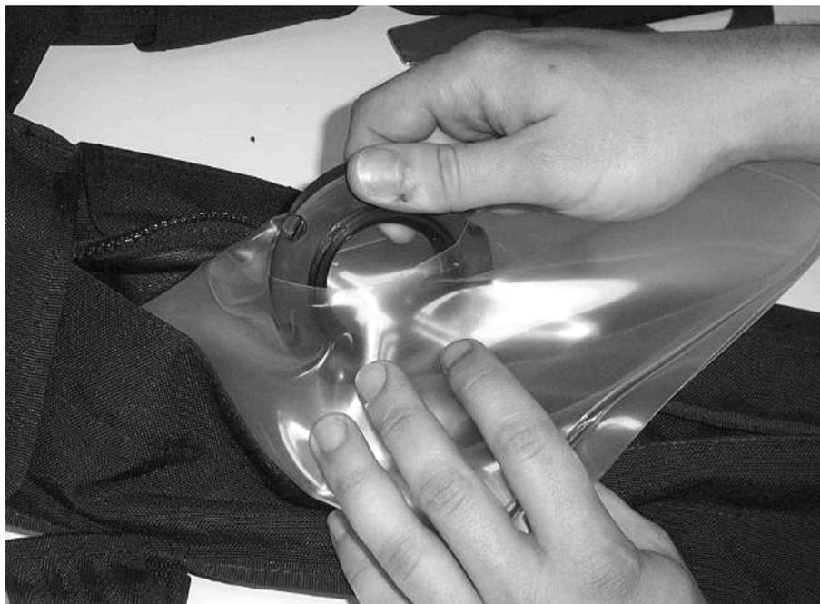
Fit the retainer base, base protector and O-ring BS130 N70 into the inner bag by placing the parts through the rear zip and into the ADV hole.
