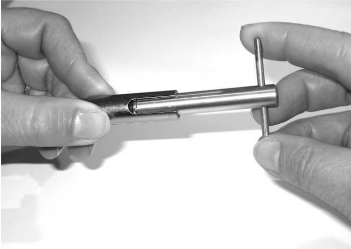
Insert the demand valve slotted tool (RB TOOL 9) into the ADV body. Make sure it connects properly into the groove on top of the tilt boss. Unscrew counter-clockwise, and take the tilt boss out of the ADV body. Make sure you do not lose the tilt axle and spring as they will now come out also.
