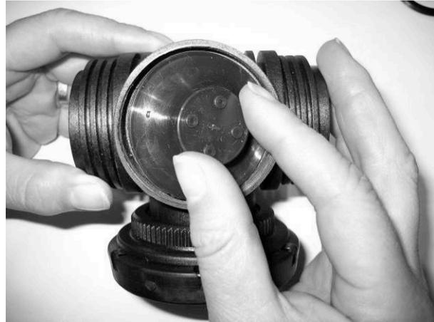
Treat the diaphragm with care. Inspect it carefully for wear and tear. Consider that damage to the diaphragm can lead to a flooded loop of your rebreather! When in doubt, replace.
