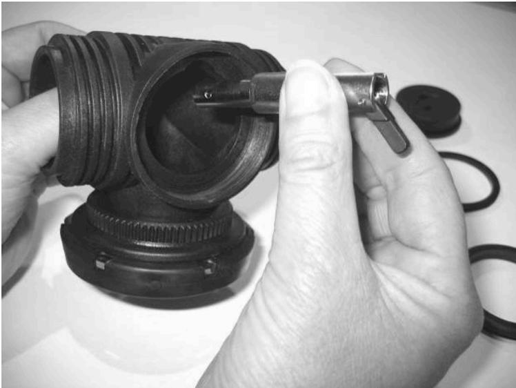
The BS014 O-ring on the outside of the banjo seals on the outer face of the ADV. Make sure you extract the ADV body carefully, without levering.
