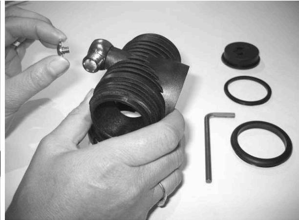
Unscrew counter-clockwise. Use a 5 mm Allen key.
