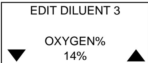
The first option is to change the oxygen percentage. Confirm by pressing the centre switch.
