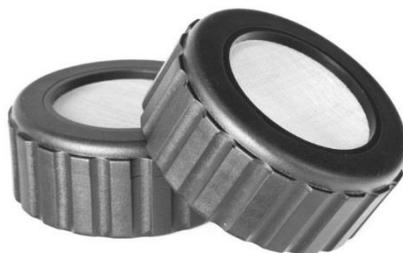
The Cell validator is supplied with “thread protection caps”, which when removed from the cell validator can be attached to the rear side of each T-piece. The caps have stainless steel mesh panels to allow the inner bags to “breathe” but also prevent insects from entering. Additional mesh caps are available separately:
