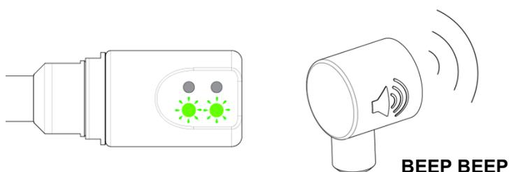
When the setpoint changes from high to low the HUD will give a double Green flash and the buzzer will give a double beep audible alarm.
