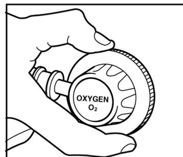
The oxygen inflator has special lubrication and seals and has undergone special cleaning to make it suitable for use with oxygen. It must only be connected to a hose supplying oxygen. As the apparatus is worn the oxygen inflator must be on the Diver's right hand, on the exhale counterlung and the diluent inflator must be on Diver's the left hand, on the inhale counterlung.
