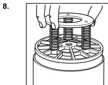
Fit the spring loaded pressure spider
