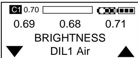
The current diluent choice is displayed. Press the left or right switch to scroll through the 12 diluents.
