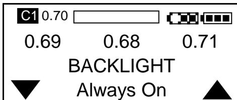
Press the right switch to get to "Always On" - a useful feature on a deep dive or in cave but remember the battery drain will be much faster and MUST be monitored closely.
