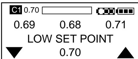
The default low setpoint is 0.70 bar but is adjustable between 0.5 and 0.9. It always defaults back to 0.7 when the electronics are turned off.
