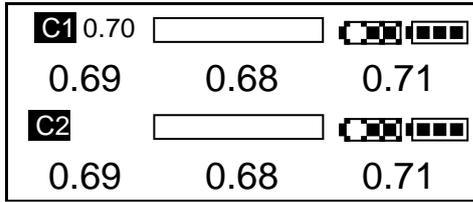
C2 can be displayed by pressing the left switch and holding for 2 secs.
