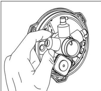
Remove the sensor by unscrewing it (anti-clockwise).
