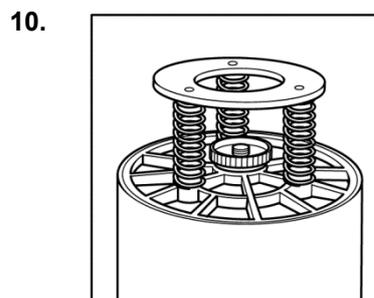
Do not over-tighten the retaining nut
