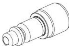
The GC5 – Gas Connector is a large bore, full flow adaptor for attaching to a male 9/16" UNF 2nd stage inlet. This allows hoses with the Auto Air type fitting (GC1A or EV50B) to be easily connected to the OCB, ADV or any 2nd stage without impeding their performance.
