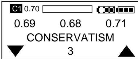
The Conservatism level is adjustable from 1 to 5, level 1 is the least conservative setting, level 2 is generally the same decompression time as level 1 but specifies a slightly deeper first stop. Level 3 is more conservative than 1, level 4 is the same as 3 but specifies a slightly deeper first stop. Level 5 specifies extra conservatism and deeper first stop.
