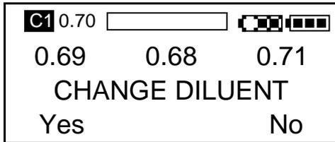
CHANGE DILUENT is a closed circuit option and is displayed if a “No” response is given to “OPEN CIRCUIT”.
