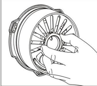
Unscrew the securing ring for the mixing chamber cover and pull the cover from the centre stem.
