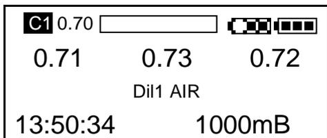
When first breathing on the rebreather, a rapid drop in ppO<sub>2</sub> will be seen. Obviously the drop in ppO<sub>2</sub> occurs because the exhaled breath contains only about 17% oxygen and you are forcing the oxygen pressure down very quickly. If you stop breathing into the loop, just take it out of your mouth, you should then expect to see the ppO<sub>2</sub> rise rapidly back towards the setpoint.
