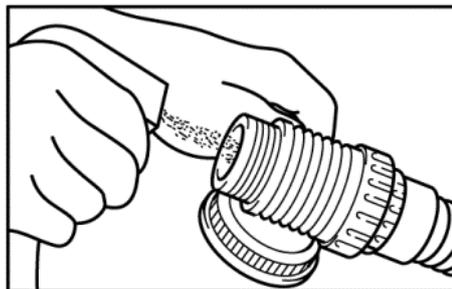
Spray or pour Chemgene HLD<sub>4</sub>L disinfectant into the T-piece
