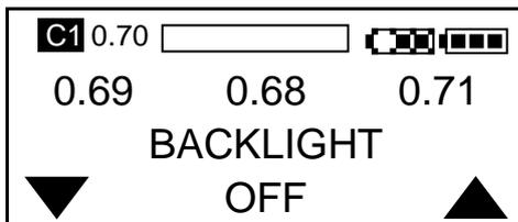
Press the down arrow once to go from "Key On" to Backlight OFF. This may be chosen in high ambient light situations to extend battery life.
