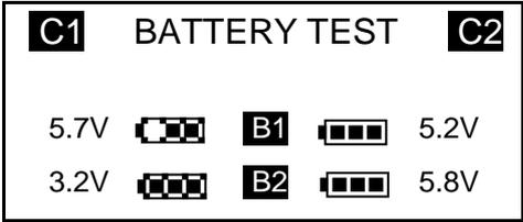
If YES is selected the battery test will commence as before. B2 may show some Voltage even if the battery is missing, this will disappear once load has been placed upon it and depleted any residual power from the capacitors.
