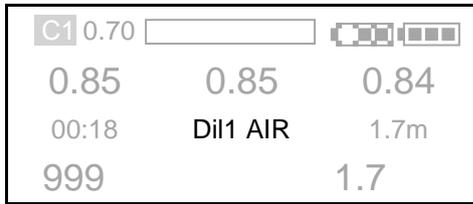
The selected diluent is shown in the centre of the display: Diluent 1, which is AIR. On the deco versions there are up to 6 diluents, all of which are user adjustable and stay in memory once set.
