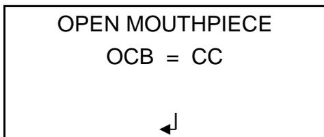
Once the oxygen percentage has been selected and confirmed by pressing the centre switch, the controller prompts OPEN THE MOUTHPIECE valve. The reason for this is to enable the cells to calibrate to ambient pressure and this would not be possible if the mouthpiece was closed.
