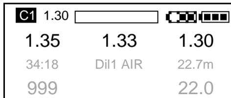
In this example the ppO<sub>2</sub> is assumed to be 1.34 bar, i.e. above the setpoint, so the solenoid will not open.
