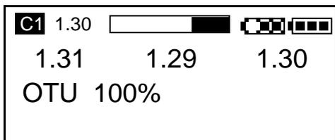
A daily OTU limit of 300 is used for the 100% indicator. A warning is raised at 100% of 300, see 3.5.6
