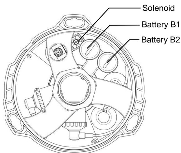
The battery life varies due to the frequency of use of the backlight and the brightness setting. To ensure that the reserve power is as good as it can be and you get the best use from the batteries always discard the batteries in B1 compartment (nearest the solenoid) when the low battery level is reached, replacing them with the two batteries from B2 and inserting new batteries into the B2 slot..
