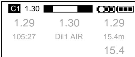
Should CO<sub>2</sub> start tracking through the scrubber this is indicated by the clear section(s) being shown between black “active” portions of the scrubber. **Abandon the dive immediately and re-pack the scrubber with fresh material.**
