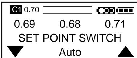
After selecting the method of changing setpoint press the centre switch to advance to the next screen.
