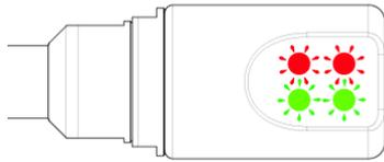
Green and red lights flashing together on C1 and C2:
