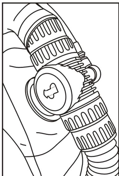
During descents it is normal for the ADV to add gas on nearly every inhalation. However, this is most abnormal during all other phases of the dive. Normally the ADV adds gas to make the counterlung volume breathable and then stops.
