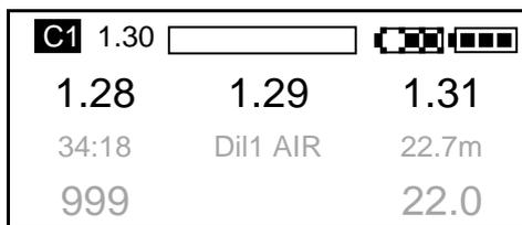
During the dive the oxygen controller controls the oxygen partial pressure in the breathing loop by averaging the nearest two cell output readings, i.e. if you have one cell reading 1.28, another 1.29 and the other 1.31, the cell displaying 1.31 will be ignored and the ppO<sub>2</sub> assumed to be 1.285. As it is below the setpoint, the solenoid will open for a fraction of a second.
