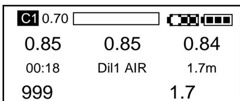
Once a depth of approximately 1.2m (4ft) has been reached, the display changes to its underwater display. It reverts back to surface display at approx. 0.9m (3ft).
