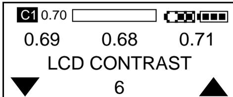
The contrast of the liquid crystal display may be altered to suit the ambient temperature. Altering the contrast has no effect on battery life. The adjustment range is 3 to 10.
