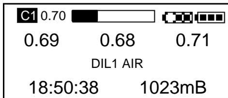
**NOTE:** When in demo mode the Scrubber monitor scrolls to indicate it is in dive mode. The left switch does not call up the Slave display (whilst in demo mode). The setpoint is automatically set at 0.21 bar and the Low Oxygen warning is set at 0.16 bar.
