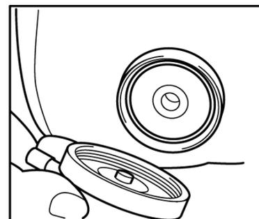
The optional rear mounted counterlungs use the low pressure, hose mounted, balanced inflators RBV05 (diluent) and RBV05A (oxygen), where the gas from the standard quick disconnect hose is fed back to the counterlungs via another LP hose.
