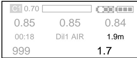
The maximum depth is shown here as 1.9m and the current depth, 1.7m, is displayed in the bottom right corner.
