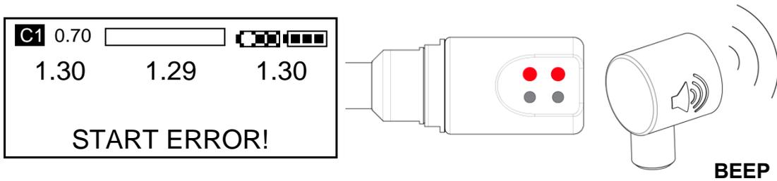
If the electronics are switched on and the pre-dive sequence is not completed and the diver enters the water, once below 1.2m(4ft) the dive Start Error will be displayed.
