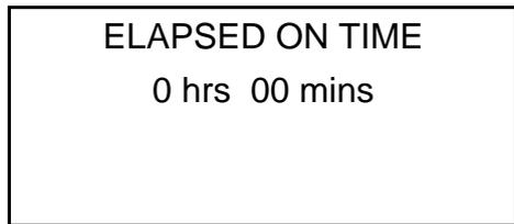
If Yes is selected then the elapsed on time is reset to zero. If No is selected then the current elapsed time is retained and the display moves to Calibration.
