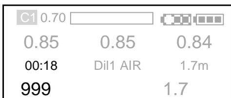
The dive time is shown, in this example, as 0 mins, 18 secs. The No-Stop time, if a decompression option is purchased, is displayed below the dive time and is shown as 999 mins.
