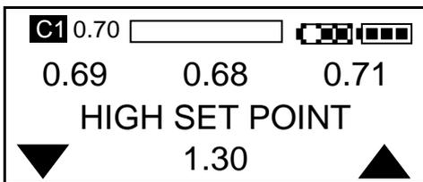
The default high setpoint is 1.30 bar but is adjustable from 0.9 to 1.5. It always defaults back to 1.3 when the electronics are turned off.
