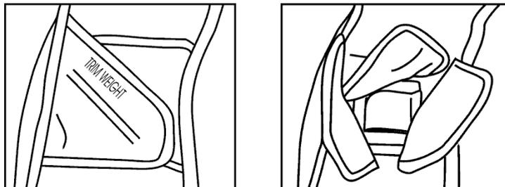
At the waist, mounted on the harness are two large weight pockets with internal removable weight pouches. To prevent un-intentional release, each weight pouch is attached with a 25mm side release buckle making it a 2-stage process to ditch the lead pouch. One pouch has a male fitting and one a female so the two pouches can be clipped together which makes them easy to carry. The weight pouches are loaded from the top through a Velcro flap and shaped with stiffeners to make loading easy.
