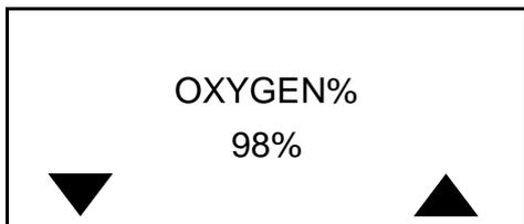
After displaying the ambient pressure value, the OXYGEN % is requested. It is requesting the oxygen % in the scrubber lid after the oxygen inject takes place during calibration.
