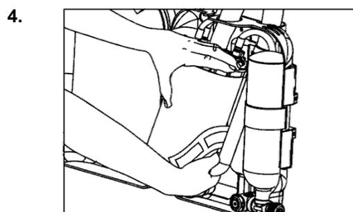
Remove scrubber hoses and electronic units from the casing
