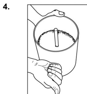
Fill to approximately half way and tap gently on the sides to level the granules
