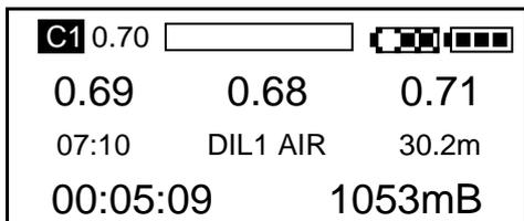
Once the shallower than approximately 1.2m (4ft) the display changes to show the maximum dive duration. Depth and a surface interval timer (hours:mins:secs) is started.
