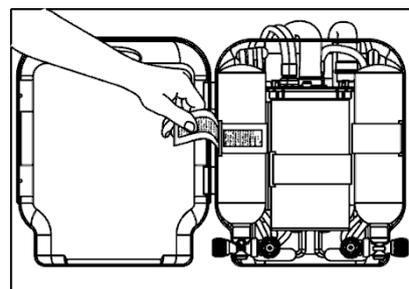
After closing the cylinder valve and purging the hoses, unscrew the DIN handwheel. If this is difficult, ensure all the pressure is released from the system. Keep this connection well lubricated using oxygen compatible grease. **DO NOT USE SILICONE GREASE OR OIL.**
