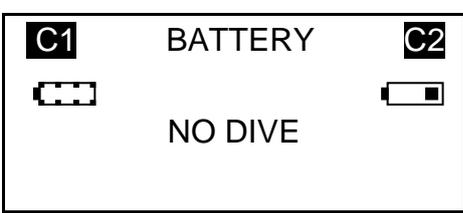
On switch on, if both batteries are displaying one icon or less - BATTERY – NO DIVE is displayed, the oxygen controller will not continue into dive mode and the dive cannot commence.
