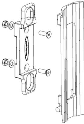
Ideal for attaching cylinders securely and conveniently to the side of the case. It features a strong and easy to operate quick release/attach mechanism. The case-plate is bolted through pre-drilled holes in the case. The cylinder plate, incorporating the quick release/attach mechanism attaches to the cylinder with rubber sleeved “jubilee” clamps (not shown). The case-plate is compatible with the range of Metalsub diving lamps and accessories.
