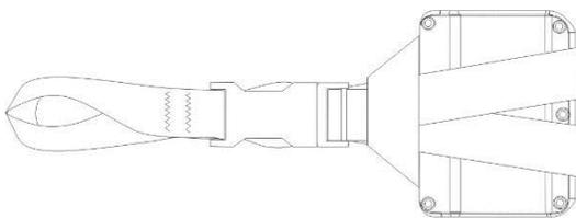
Normally the display is mounted on the diver’s wrist retained by the two wrist straps. Alternatively, a display strap can be used to suspend the display, attached to a suitable D ring with a quick release buckle.
