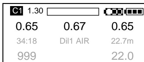
In this example the ppO<sub>2</sub> is assumed to be 0.65 bar, which is a long way below the setpoint, so the solenoid will open for a number of seconds.
