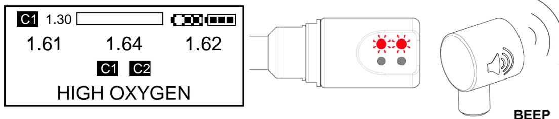
The HIGH OXYGEN warning is set at 1.6 bar. One or both red lights flash **quickly**, the buzzer sounds and “HIGH OXYGEN” is displayed alternating with  $ppO_2$ , depth and dive time information. The warnings will continue until the  $ppO_2$  drops below 1.6 bar.
