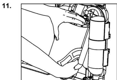
The scrubber locates on the back frame and is held in place by the Velcro band. The inlet pipe MUST sit underneath the cylinder against the back-frame.
