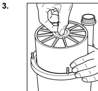
Remove the cartridge using the moulded centre stem.
