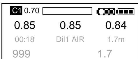
The top two lines are the same as the Dive Mode – Surface. The ppO<sub>2</sub> detected by the oxygen cells is displayed across the centre of the display.
