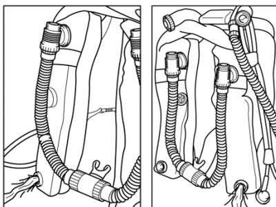
Repeat the process, thoroughly flushing the counterlungs with fresh water
