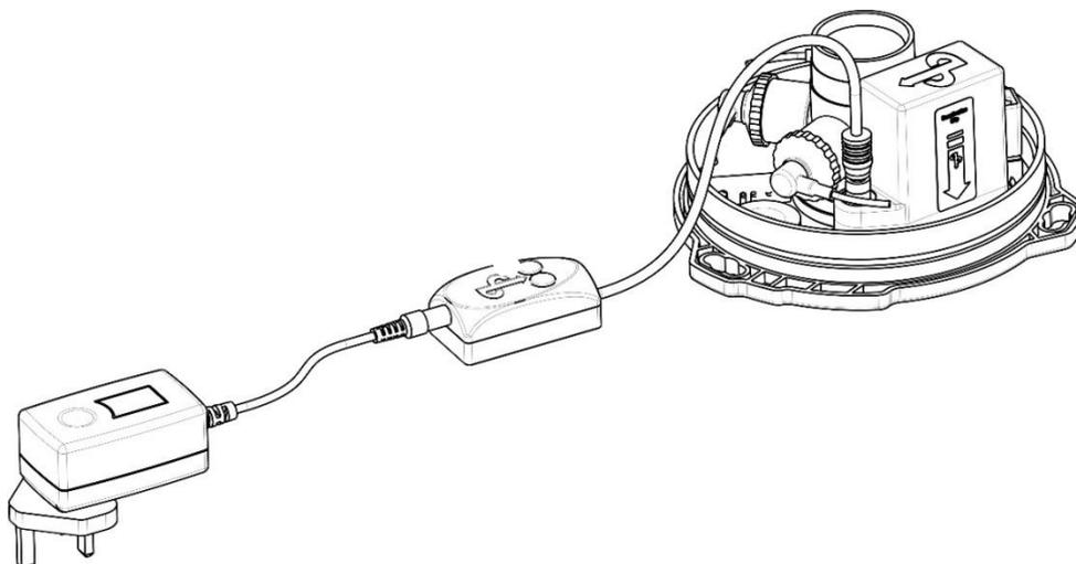
6. The dual charger will light up showing the charge status of each battery within the battery pack.
