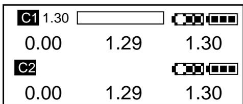
In this case the problem is seen by both controllers, which indicates a faulty cell connection or faulty cell.
