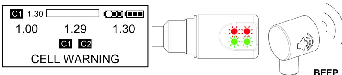
A CELL WARNING occurs if one cell deviates from the average of the closest two by more than 0.2 bar.
