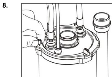
Lift and turn each catch to lock the lid in position
