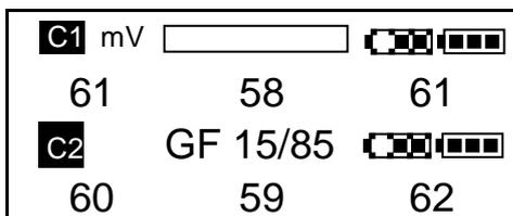
Left Switch, 4 second hold – displays the raw cell readings in mV, at a resolution 1 mV.
