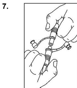
Carefully disconnect scrubber monitor cable and only fit protective covers when dry.
