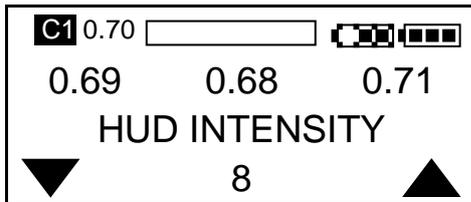
The intensity of the head up displays' LEDs may be altered to suit the ambient light. A night dive may require a lower intensity. Adjustment range is 1 to 10.
