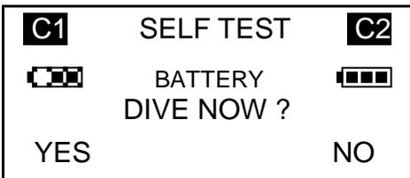
When switching on, if one battery is down to one icon (approx. 5.2 volts) and the other battery has two or three icons a warning screen appears which requires a YES or NO decision to continue the dive. It is recommended that if a near the limits dive is planned, or if the apparatus had been stored at a low temperature, the battery should be replaced.
