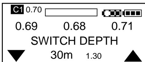
The switch from LOW setpoint to High setpoint can be set to take place automatically by selecting AUTO and is preferable to using “Manual” (See section 1.7). The next screen allows you to select the switch depth. Whatever depth you set it to will be remembered the next time you switch on. Press the centre switch to select the depth and move to the next menu option.
