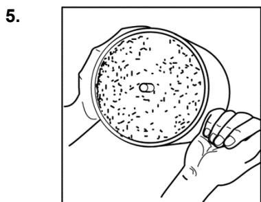
Fill to within 6mm of the top and tap gently on the sides to level the granules
