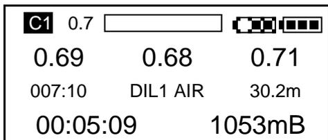
Missed Deco will be displayed on the screen if the diver surfaces without decompressing according to the dive computer. This is alternated with DOWN and the Surface Interval information.
