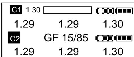
Left Switch, 2 second hold – displays the Slave's ppO<sub>2</sub> and battery readings on the bottom two lines of the display. The Gradient Factors are displayed in the centre of the screen (Trimix Version only).
