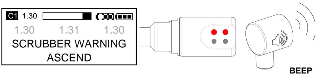
The final scrubber warning is given when the active area of the scrubber is too small to remove the CO<sub>2</sub> effectively. This is shown on the scrubber monitor as a blank screen. The warning is not suppressible. You must ascend and revert to open circuit bailout.
