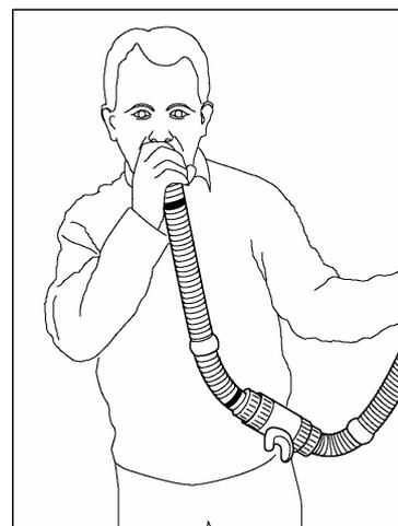
A head strap can be fitted to the mouthpiece valve assembly which offers additional support by holding the mouthpiece towards the wearer. The strap is particularly useful on long duration dives by minimising the effort needed to retain the mouthpiece in position, thereby reducing jaw fatigue. A head strap may also help retain the position of the mouthpiece if the diver becomes unconscious.
