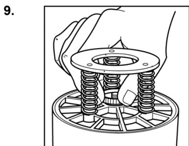
Fasten the retaining nut
