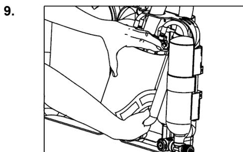
When re-inserting the scrubber assembly ensure the Velcro band passes between the scrubber wall and the down pipe
