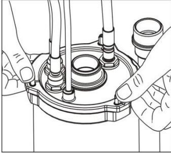
To replace the oxygen cells it is necessary to remove the scrubber from the rebreather.
