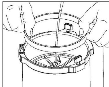
Ensure the spacer ring is clean and undamaged and place carefully onto the O ring. Again push down and ensure the cartridge is free to move up and down and check for the spring loading effect of the pressure spider. If the spacer ring is marked on one side, turn it over to ensure the good side sits on the O ring. Should both sides of the spacer be marked, replace the spacer with a new one before diving.
