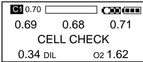
The Cell Check Screen shows what the PPO<sub>2</sub> displays should be, if the loop is flushed properly at the current depth with diluent or oxygen. Cell Check is displayed for 15 seconds. If a switch is not selected within 15 seconds the display will revert to Dive mode display.
