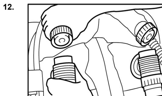
Re-fasten the hoses. Nip them up hand tight. Excessive force does not improve the sealing effect so DO NOT over-tighten.
