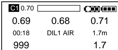
Once the pressure is equivalent to approximately 1.2m (4ft) the display enters the underwater mode.
