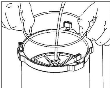
Ensure this O ring is undamaged, clean, lightly lubricated and properly located. Also check for any dirt or damage on the top of the cartridge and place the O ring on top.
