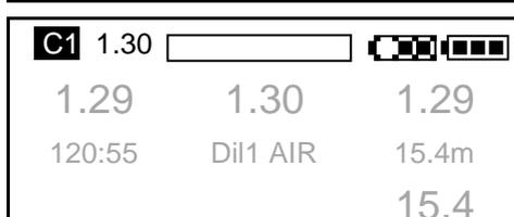
The scrubber monitor simply shows the active part of the scrubber. The gauge starts out empty and as the bottom of the scrubber warms up, the display on the left side of the scrubber display turns black, followed by the next segment and so on progressing across the scrubber monitor from left to right.
