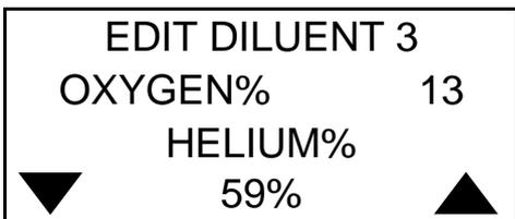
Next, it is possible to adjust the Helium %. If Heliox were being used then increase the Helium % to eliminate any Nitrogen.
