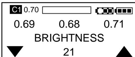
The backlight is the 2<sup>nd</sup> biggest power consumer. The maximum setting is 31. By setting this to 21 there is a saving of 30mA. Press the centre switch to select. Adjustment range is 1 to 31; the lower the number the lower the current-drain on the batteries.
