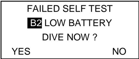
This warning screen shows battery B2 as low or missing. If YES is selected to DIVE NOW the Battery Test Screen will appear as before. A further warning screen will appear after the solenoid “load” test has been conducted.
