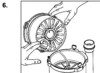
Ensure the bottom lip on the canister lid is undamaged, clean and properly located. Tuck the excess cable and connector into the lid spacer.
