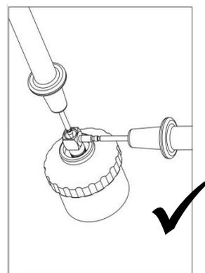
3. If you need to measure the output voltage of the oxygen cell, attach a spare connector to the cell and place your DVM (Digital volt meter) probes on the connector. The central pin is +ve and the exterior of the connector is -ve.
