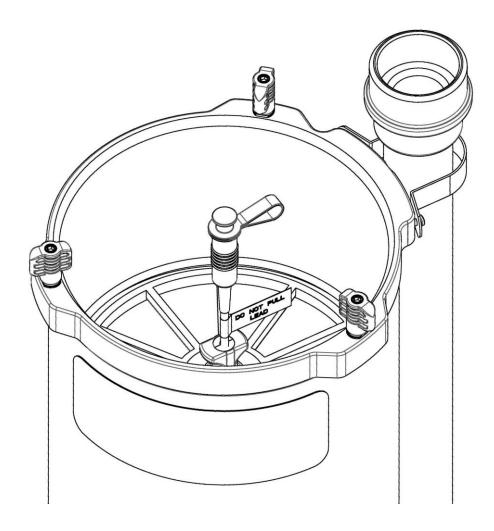
5. Assemble the lid into the canister and complete the rebreather setup as normal including all the pre-dive checks.
