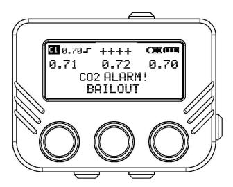
The  $CO_2$  Sensor will trigger an alarm when  $CO_2$  reaches 5mbar in the breathing loop. The display will show " $CO_2$  ALARM! BAILOUT". This will cycle with any other warnings that might be present. The warning will also be shown on the Vision HUD, whilst the buzzer sounds. The HUD will show solid red lights on both controllers for the period that the  $CO_2$  is above 5mbar.
