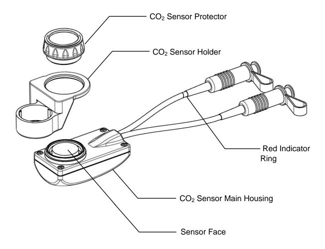
Note: Take care not to damage the Sensor face itself or leave this exposed. Always store the sensor with a used  $CO_2$  Sensor Protector assembled onto it as protection. Before use you should make sure that the sensor face is free from moisture as this can affect the sensors accuracy in use.
