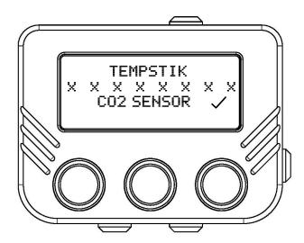
However, should the  $CO_2$  sensor not be detected, the  $CO_2$  sensor is simply not shown:
