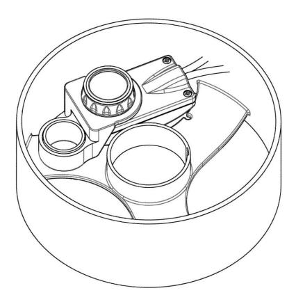
3. The mixing chamber is then placed onto the lid and secured by the mixing chamber locking ring as normal.
