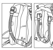
Repeat the process, thoroughly flushing the counterlungs with fresh water
