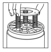
Remove the spring/ pressure plate assembly
