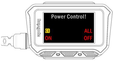
Here the option is given to either switch off completely by selecting ALL or switch on C1.
