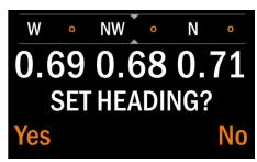
This displays the 'SET HEADING?' option. Pressing the left button to select 'Yes' will set your current direction as a heading, by placing a marker on the inner band of the compass.
