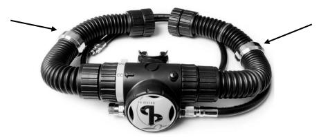
The hose weights should be moved to ensure the mouthpiece sits horizontally, has neutral buoyancy and sits comfortably in your mouth. e.g. If the mouthpiece is digging into your top lip, either the hoses are twisted or the mouthpiece is too buoyant, in which case moving the hose weights towards the mouthpiece ensures better comfort. Conversely, if the mouthpiece is too heavy, move them outwards.
