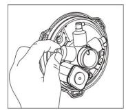
Remove the blue connector covers and pull the cell connector from the cell (straight pull).
