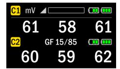
The oxygen sensor mV readings and gradient factor details can be seen by keeping the left button held for a further 2 seconds.
