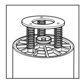
Do not over-tighten the retaining nut
