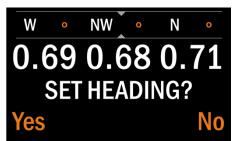
Selecting 'Yes' by pressing the left button would set a new heading (replacing a current one if it had been previously set), but selecting 'No' by pressing the right button will give the option to turn the compass off:
