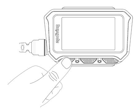
The two controllers perform their self-tests. C1 performs its test first and if the connection to the display is operational the display backlight will come on and the start-up splash screen is displayed.
