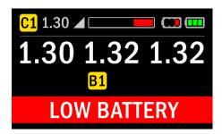
Whenever a warning is active on the display, the top bar information will be shown along with the warning but the compass details will still be shown as the warning alternates with the depth, time and decompression information.
