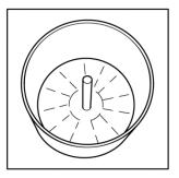
The filter scrim must be located properly in the bottom with no gaps around the edges or the centre column. Its purpose is to retain the Sofnolime granules and keep water out
