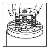
Fit the spring loaded pressure spider
