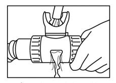
Spray the mouthpiece with disinfectant and thoroughly flush through.
