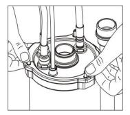
To replace the oxygen cells it is necessary to remove the scrubber from the rebreather.
