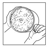
Fill to within 6mm of the top and tap gently on the sides to level the granules
