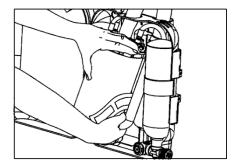
Remove scrubber and connected hoses from the casing
