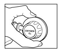
The oxygen inflator is located on the exhale lung, on the diver's right hand side. The diluent inflator is located on the inhale lung, on the diver's left hand side. The oxygen inflator is cleaned and lubricated with oxygen compatible grease. The oxygen inflator must only be connected to oxygen hoses to prevent cross contamination.
