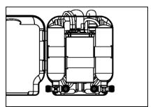
Location of cylinders and 1<sup>st</sup> stages inside the case.
