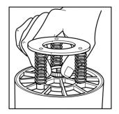
Turn the cartridge over and unscrew the retaining nut
