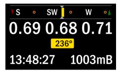
In this first example the small green arrow on the right of the compass band shows you would turn to the right to return to the original heading and the small red arrow on the left that you would turn to the left to follow the reciprocal heading.
