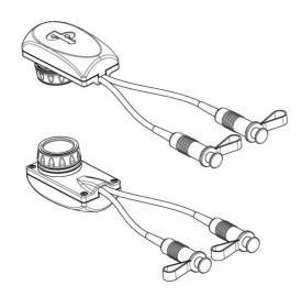
For this reason, the AP CO<sub>2</sub> Sensor utilises a drying cartridge that consists of a desiccant sandwiched between protective technical membranes to prevent water vapour interfering with the detection of CO<sub>2</sub>. The effect of pressure on the CO<sub>2</sub> Sensor is compensated for with a complex software algorithm. This enables the output of the sensor to be corrected according to changes in pressure experienced during diving.
