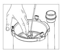
Push down and ensure the cartridge is free to move up and down and check for the spring loading effect of the pressure spider
