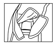
At the waist, mounted on the harness are two large weight pockets with internal removable weight pouches. To prevent un-intentional release, each weight pouch is attached with a 25mm side release buckle making it a 2-stage process to ditch the lead pouch. One pouch has a male fitting and one a female so the two pouches can be clipped together which makes them easy to carry. The weight pouches are loaded from the top through a Velcro flap and shaped with stiffeners to make loading easy.
