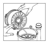
Ensure the bottom lip on the canister lid and Lid Oring are undamaged, clean and properly located. Tuck the excess cable and connector into the lid spacer.
