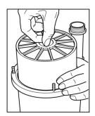
Remove the cartridge using the moulded centre stem.
