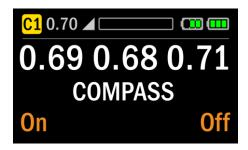
In Surface or Dive Mode, the compass can be accessed by holding the right button for 2 seconds, then press the left button.
