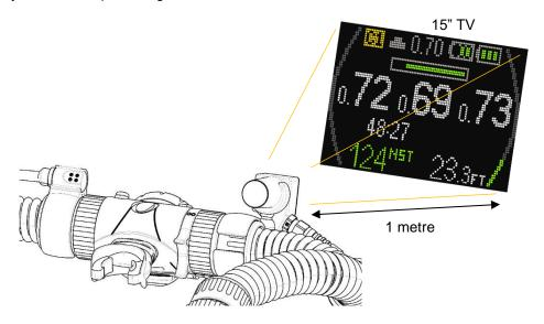
The HUS is compatible with all AP Diving rebreathers equipped with Vision electronics - programmed with V06.00.00 firmware or later.
