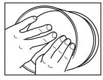
Ensure the filter scrim is clean and undamaged. Push in into the cartridge as far as it will go.
