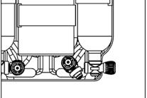
After closing the cylinder valve and purging the hoses, unscrew the DIN handwheel. If this is difficult, ensure all the pressure is released from the system. Keep this connection well lubricated using oxygen compatible grease. DO NOT USE SILICONE GREASE OR OIL.
