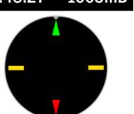
The heading is shown as a green arrow on the inner band. As you change direction the marked heading will scroll with the cardinal points on the inner band, giving an indication of which way to turn to get back to your original heading.
