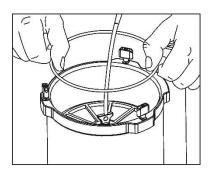
Ensure the Oring is undamaged, clean, lightly lubricated and properly located. Also check for any dirt or damage on the top of the cartridge and place the O ring on top.
