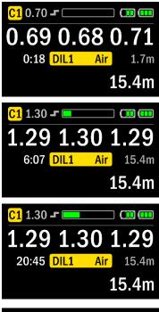
The scrubber monitor simply shows the active part of the scrubber. The gauge starts out empty and as the bottom of the scrubber warms up, the display on the left side of the scrubber display fills, followed by the next segment and so on progressing across the scrubber monitor from left to right.
