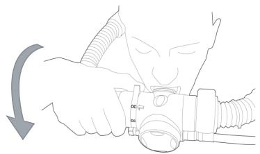
The two modes are selected by rotating the lever forwards or backwards, which in turn rotates the internal components within the main body. The Rebreather mode is activated by rotating the lever to the backward position where the lever is in line with the mouthpiece. The Open circuit mode is activated when the lever is rotated forward to the 'up' position.
