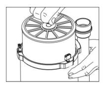
After inspecting the bore for damage or dirt - Insert the cartridge carefully taking care not to scratch any components
