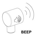
A CELL WARNING occurs if one cell deviates from the average of the closest two by more than 0.2 bar.
