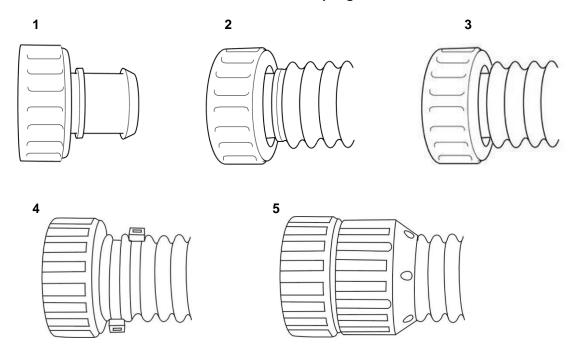
1, 2 & 3: Push the coupling into the hose until the hose is against the shoulder of the fitting. NOTE:
