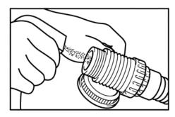
Spray or pour Chemgene HLD<sub>4</sub>L disinfectant into the T-piece
