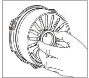
Unscrew the securing ring for the mixing chamber cover and pull the cover from the centre stem.
