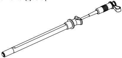
The central rod of the scrubber is replaced by the 'Tempstick', a similar rod with internal temperature sensors, connected by a cable. This is a plug and play device. Inside the scrubber lid is a spare connector: connecting this to the corresponding connector on the temperature stick activates the software so the scrubber monitor is shown in the top centre of the wrist-mounted display.
