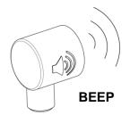
**NOTE:** The Scrubber warning system does not measure CO<sub>2</sub>, it monitors scrubber activity by measuring the temperature throughout the Sofnolime bed.
