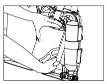
When re-inserting the scrubber assembly ensure the Velcro band passes between the scrubber wall and the down pipe
