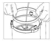
Ensure the spacer ring is clean and undamaged and place carefully onto the O ring. Again push down and ensure the cartridge is free to move up and down and check for the spring loading effect of the pressure spider. If the spacer ring is marked on one side, turn it over to ensure the good side sits on the O ring. Should both sides of the spacer be marked, replace the spacer with a new one before diving.
