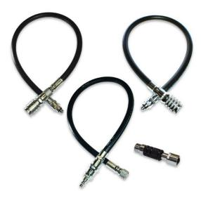
The heart of the gas connection system (GCS) consists of 2 quick release hose fittings, one male and one female. The hose with the male fitting connects to the **ADV** or 2nd stage and the female connects to the intermediate (low) pressure port of your 1st stage.
