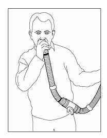
A head strap can be fitted to the mouthpiece valve assembly which offers additional support by holding the mouthpiece towards the wearer. The strap is particularly useful on long duration dives by minimising the effort needed to retain the mouthpiece in position, thereby reducing jaw fatigue. A head strap may also help retain the position of the mouthpiece if the diver becomes unconscious.
