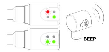
A low battery warning is indicated by alternating red/green/red/green etc flashing lights in C1 or C2 or both if both have low battery levels.
