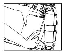
The scrubber locates on the back frame and is held in place by the Velcro band. The inlet pipe MUST sit underneath the cylinder against the back-frame.
