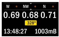
The compass band and direction in degrees then replaces the top line information and the diluent gas respectively. The top line information and diluent can be seen at any time whilst the compass is active by holding the left button for 2 seconds.
