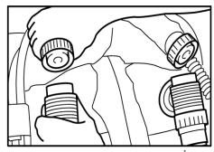
Re-fasten the hoses. Nip them up hand tight. Excessive force does not improve the sealing effect so DO NOT over-tighten.
