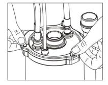
Remove the lid by pulling upwards
