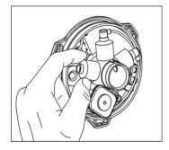
Remove the sensor by unscrewing it (anti-clockwise).
