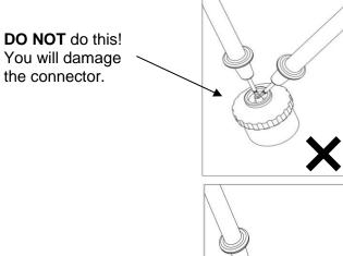
If you need to measure the output voltage of the oxygen cell, attach a spare connector to the cell and place your DVM (Digital volt meter) probes on the connector. The central pin is +ve and the exterior of the connector is -ve.
