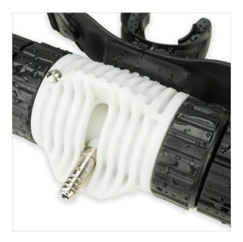
The photograph above shows the underside of the mouthpiece valve showing the operating lever and the two moulded-in flanges which allow one handed operation. The rotational inner and outer body are injection moulded in a PTFE filled, self-lubricating, acetal polymer. The slotted lock screw, top left, prevents accidental unscrewing of the blue inhale-valve-holder (not visible). The operating lever, made in nickel-plated-brass, screws into a moulded-in brass-threaded-insert for added strength.
