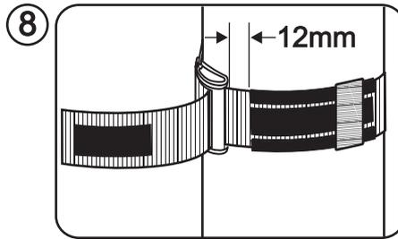
8 Ensure that the rubber sleeve does not interfere with the buckle.
