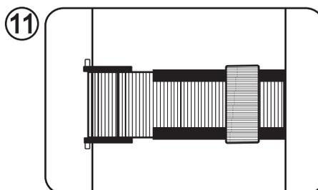
11 After securing the cylinder, check that the belt is sitting straight and firmly.
