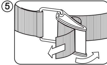
5 Secure the webbing by pulling the buckle slightly forward. Now thread the remaining webbing through the buckle as shown.
