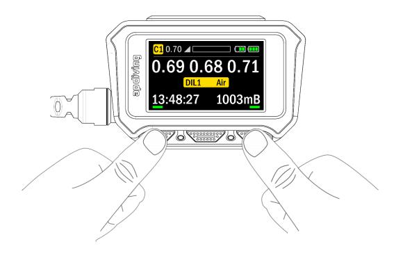
To enter or exit MENU Mode, press the outside two buttons simultaneously or within 0.5 seconds of each other.
