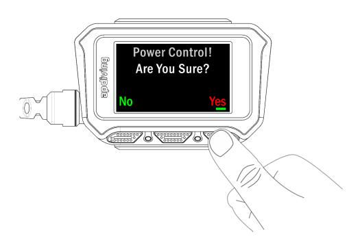
The Power Control allows the shutdown of either of the controllers or the whole system, except when underwater.
