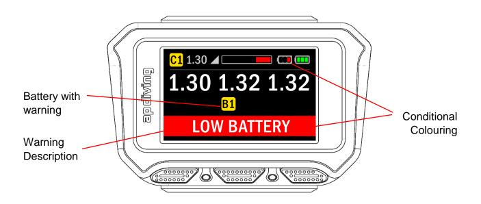
The 2020 Colour Display shows which Controllers (or Batteries) are generating the warning and the warning is displayed in high contrast white on red.
