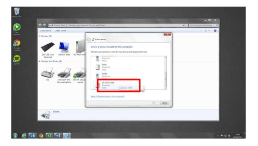
4. Often the device is automatically paired but on some systems, particularly MACs, you will be required to enter the "device's pairing code", which is *apvision* (all in lowercase, no spaces). This will pair the Vision electronics with the computer and it will now be displayed in the 'Devices' of the 'Devices and Printers' window.
