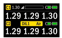
The top line controller 1 information, controller 2 information and diluent can be seen at any time whilst the compass is active by holding the left button for 2 seconds.
