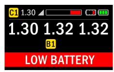
Whenever a warning is active on the display, the top bar information will be shown along with the warning but the compass details will still be shown as the warning alternates with the depth, time and decompression information.
