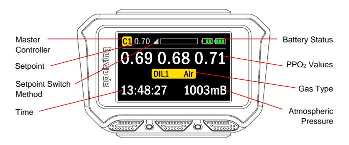
The 2020 Colour Display has been laid out in a very similar fashion to the previous monochrome display so it is very easy for existing users to switch between the two displays.
