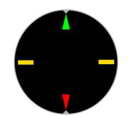
When a heading is set with a green arrow marker, 3 other markers are placed on the inner band at the same time. A red inverted arrow is placed at 180 degrees to the heading as a reciprocal marker and two yellow rectangular markers are also placed at 90 degrees to the heading. These are useful references when swimming perpendicular to the heading marker, for instance during a square search or to simply move along the reef.
