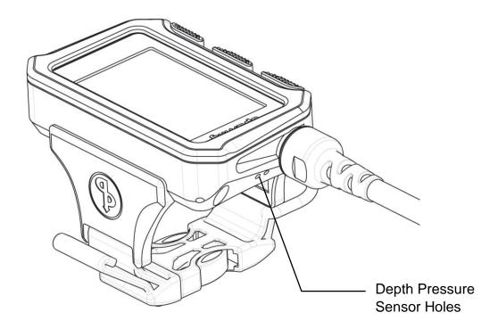
**Note:** Make sure that the depth pressure sensor holes are not impeded in any way that could affect their use
