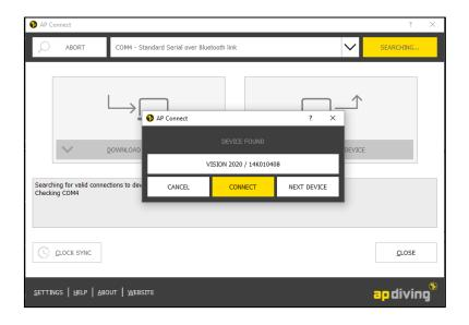
8. If the link is successful the yellow box in the top right corner will display "CONNECTED" and the "DOWNLOAD FROM DEVICE" and "UPLOAD FROM DEVICE" icons will be highlighted.
