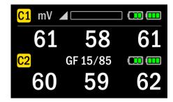
The oxygen sensor mV readings and gradient factor details can be seen by keeping the left button held for a further 2 seconds.
