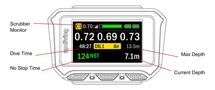
The no stop time is shown in green, meaning there is currently no decompression required. The scrubber monitor and battery status are also in green showing a good condition. All other information in this example is shown in white and grey as they are all within the appropriate limits.
