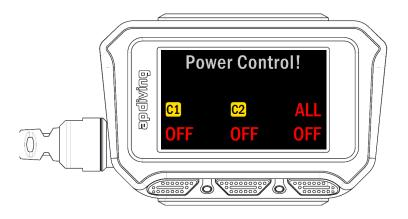
Whilst underwater you cannot turn off the entire system, the ALL OFF option shown at the surface becomes NONE OFF. If one controller is switched off it may be switched on again using the same power control screen.
