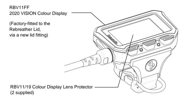
The 2020 Colour Display comes factory-fitted to the Rebreather Lid. It is wired into the controllers via a new flexible cable assembly. The rebreather firmware must be V07.00.00 or higher for the Colour Display to work and this will be installed as standard.
