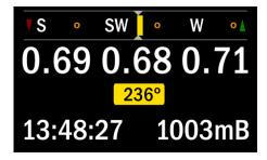
With a heading set, the compass features two heading indicators to show which way to turn to return to the original heading, reciprocal or 90 degree marker.
