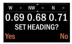
This displays the 'Set Heading?' option. Pressing the left button to select 'Yes' will set your current direction as a heading, by placing a marker on the inner band of the compass.
