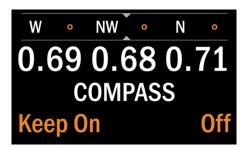
Selecting the right button turns the compass off. Any set heading markers are still retained and displayed when the compass is turned on again. The heading markers are lost though when the handset is powered down and it will be necessary to reset heading markers prior to the next dive.
