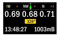
The heading is shown as a green arrow on the inner band. As you change direction the marked heading will scroll with the cardinal points on the inner band, giving an indication of which way to turn to get back to your original heading.
