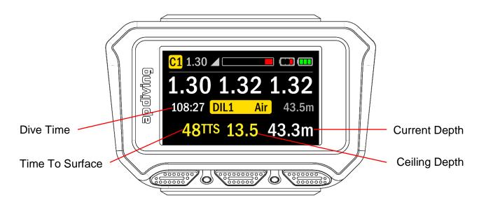
The time to surface and ceiling depth are shown in yellow, highlighting the decompression obligation currently in place. The scrubber monitor and B1 battery status in this example are in red showing a low battery issue and poor condition of the CO<sub>2</sub> scrubber.
