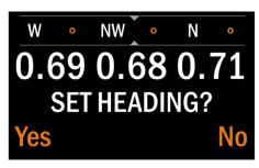
Selecting 'Yes' by pressing the left button would set a new heading (replacing a current one if it had been previously set), but selecting 'No' by pressing the right button will give the option to turn the compass off:
