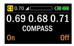
Once within Surface or Dive Mode, the compass is accessed by holding the right button for 2 seconds. Pressing the left button then turns the compass on and pressing the right button continues with the compass off.
