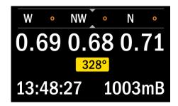
Once the compass is activated a heading can be set by holding the right button for 2 seconds
