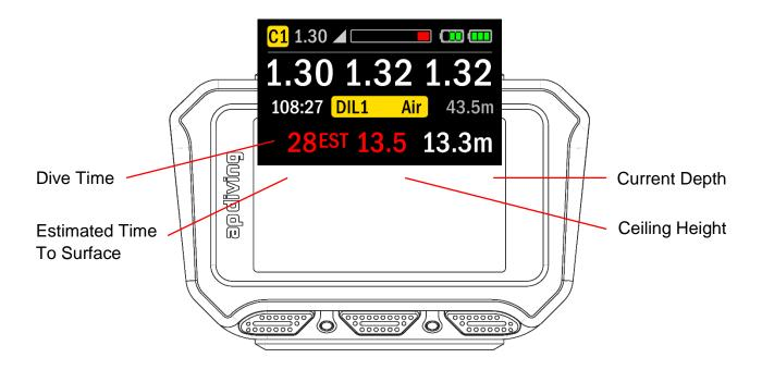
The estimated time to surface and ceiling depth are shown in red, highlighting the fact that the decompression is now estimated due to the ceiling violation.
