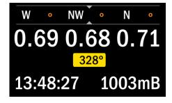
The compass band and direction in degrees then replaces the top line information and the diluent gas respectively. The top line information and diluent can be seen at any time whilst the compass is active by holding the left button for 2 seconds.
