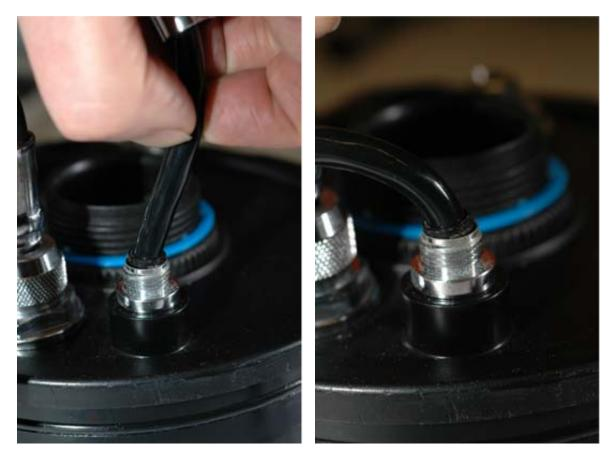
Slide the cable collet up the cable:
