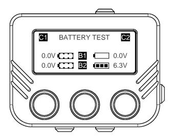
In this scenario, B1 has insufficient voltage and, as there is no B1- there is no C1 (Controller 1). C1 cannot measure anything, as it's not switched on, so 0.0v is displayed for both B1 and B2 in the C1 column. C2 is working properly and reports 6.3v for it's own battery (B2) and 0.0v for B1.
