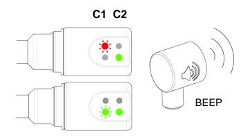
A low battery warning is indicated by alternating red/green/red/green etc flashing lights in C1 or C2 or both if both batteries are low.
