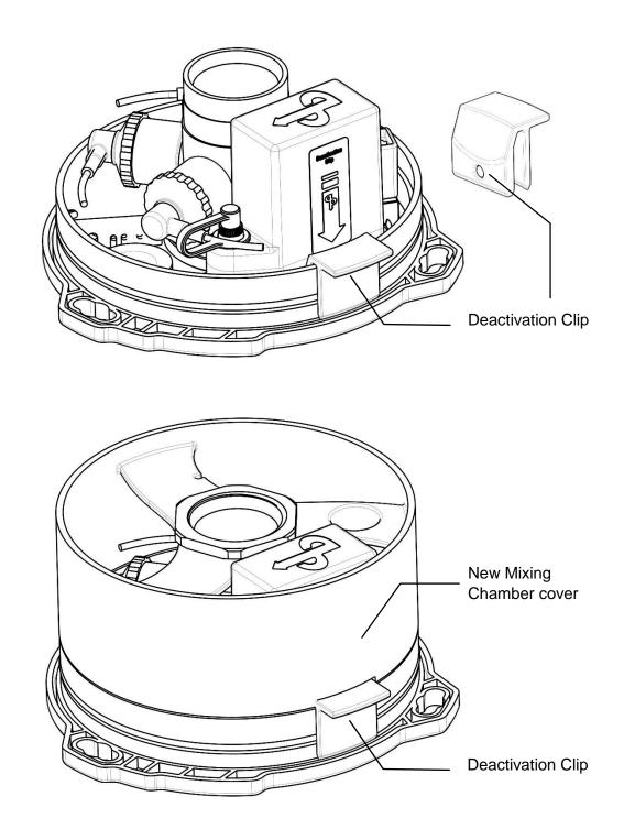
This clip allows the diver to isolate the power supply when flying with the rebreather lid and also avoid the worry of the auto activation turning the unit on unnecessarily when in a damp environment.
