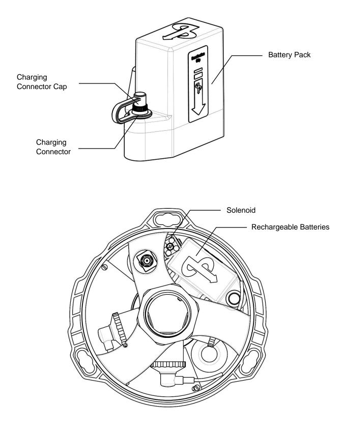
Note: The Rechargeable batteries are hardwired into the rebreather controller and as such are not user removable, but can be deactivated using the deactivation clip.
