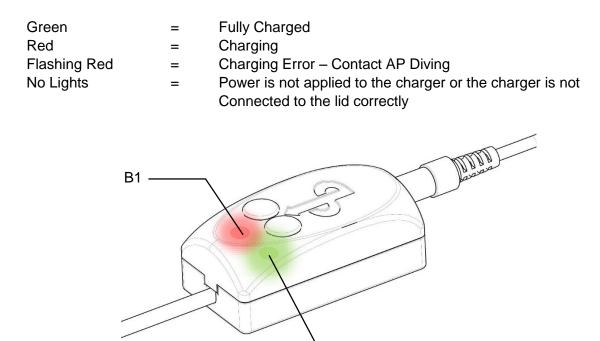
The image here shows B1 charging and B2 fully charged. When both B1 and B2 show green the batteries are fully charged and ready for use.
