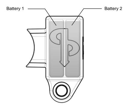
If B1 is discharged, there will be no C1 controller, the same applies for B2 & C2 – no battery, no controller. If there is sufficient charge in B1 for all operations it will automatically be used as the Master battery. If B1 only has sufficient power to start the C1 processor, C1 will still be the Master oxygen controller but B2 will be promoted to the Master battery status and will be used for powering the solenoid, wrist display and HUS if fitted.
