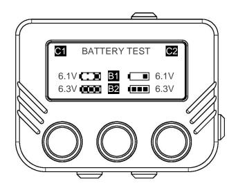
If one battery reading is low, one or zero squares, and the other battery has two or more squares the "SELF-TEST, BATTERY, DIVE NOW YES OR NO?" screen will appear.
