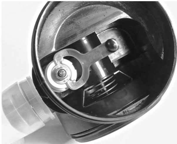
WRONG: Legs of breathing module are NOT facing diaphragm and hose
