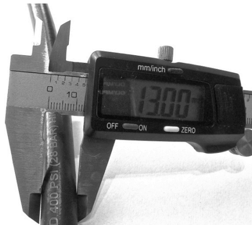
New standard type 13 mm diameter MP hose
